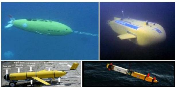
Fig. 6. Torpedo shaped AUV [1]
