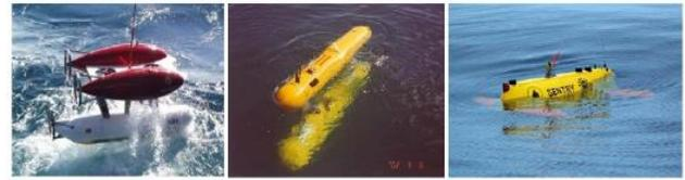
Fig. 7. Non-torpedo shaped AUV [1]
