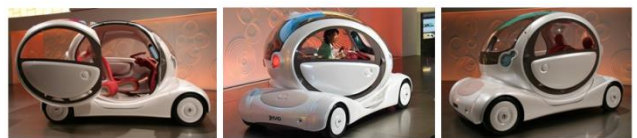
Fig. 3. Nissan Pivo; ability to rotate 360 degree due to the advance technology used for power train
