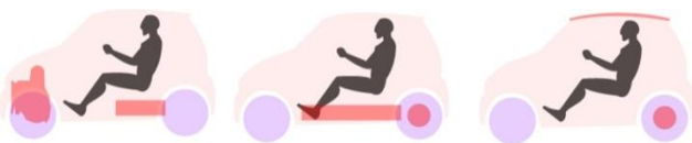
Fig.6. The comparison of powertrain between the ICV (left) and the BEV (Middle) and Solar (right).
