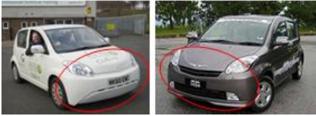
Fig.9. The differences of the front end between EV Avid Cue-V (left) and ICV Perodua Myvi (right)
